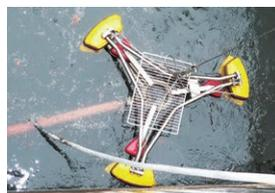
Polyethylene pellet collection equipment at UBE Elastomer Co. Ltd.
