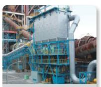
This facility uses a chlorine bypass system, achieving a high bypass ratio
