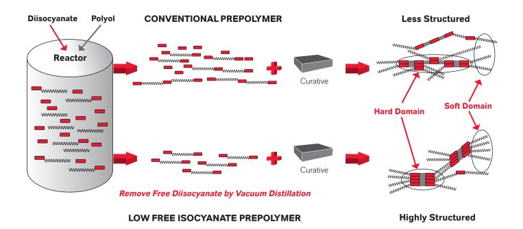
Adiprene<sup>®</sup> LF prepolymers have a highly structured morphology to provide superior performance, including excellent toughness, fatigue resistance, and longer lifetimes when exposed to extreme conditions of temperature and chemicals. They are used in a diverse range of adhesives and sealant applications in construction, automotive, electrical, and packaging.
